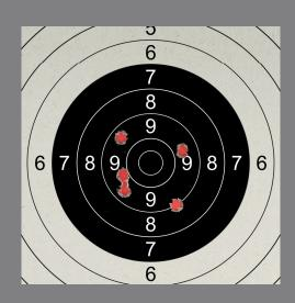
The APC223 produces excellent accuracy. The precision from a supported position can put all the rounds of a five-round test group into the 9 ring circle at 100 meters. That is a group of about 28 mm (1.1 Inch) and is more than sufficient for any normal dynamic competition. As a matter of fact it is better than many other .223 weapons in
